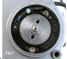
Step 11 The timing can be easily set with the piston at TDC (Top Dead Centre), then by rotating the pulser ring, align the correct full advance setting, as engraved on the ring, with either line on the rotor. Example shown in Fig. 3 is set at 28° for a 450cc engine. This setting can be checked with a strobe light when the engine is running. The line on the rotor should be seen to align with the 'FA' engraved on the ring as rpm is increased.
