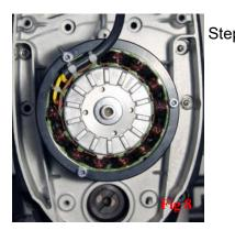
Step 4. Fit the rotor onto the shaft using the original bolt and large washers provided see Fig 8. Tighten bolt to specified torque. Check the rotor is not touching the stator, there must be a small air gap of approx. 0.5mm between the rotor and stator, this can be checked by inserting a slip of paper.
