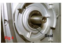
alternator fitted. For this type the original crankcase seal, in the timing cover, needs replacing with one of 28x38x7. If this seal is required please contact us and we can send one free of charge.
